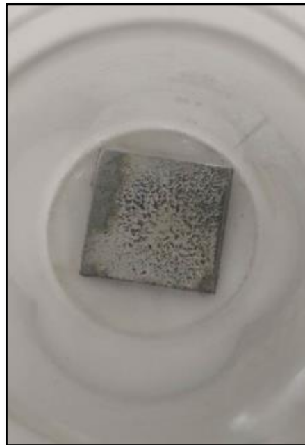
Figure III.21: results of coating with 7.5mg concentration TiB 2 of ethanol
