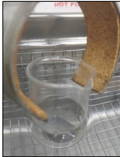
Figure III.13: method of immersion the sample assisted by ultrasonication .
