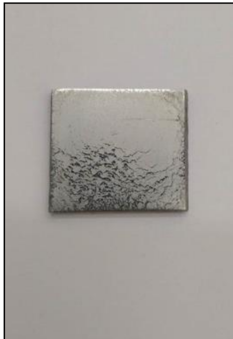
Figure III.17: coating surface with 5mg of TiB 2 powder results by laboratory oven
