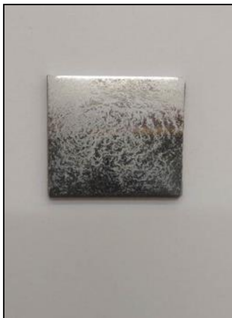
Figure III.19: coating surface with concentration 1 mg \text{TiB}_2 powder mixed with 5 ml of water
