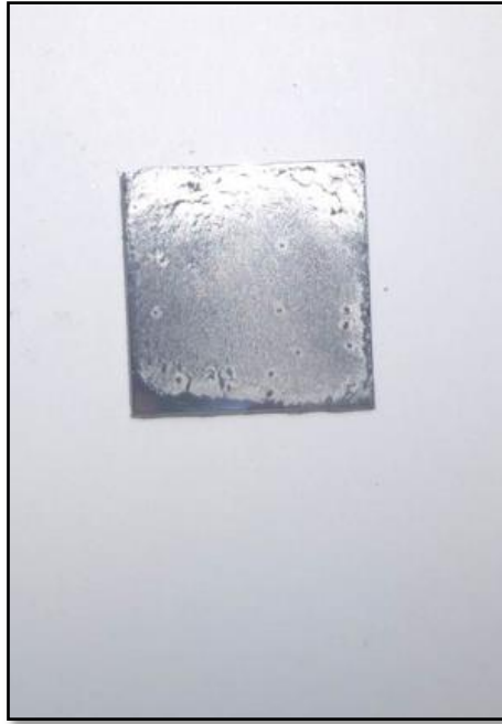
Figure III.16: coating surface with 7.5mg TiB 2 powder results by laboratory oven
