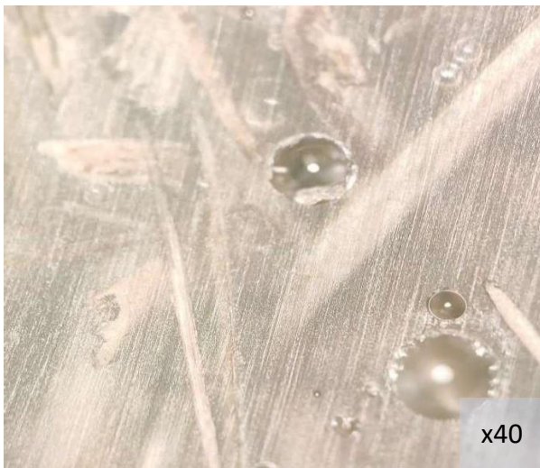
Figure III 5 microstucture du composites alpha+epoxy vieillie a 40°C
