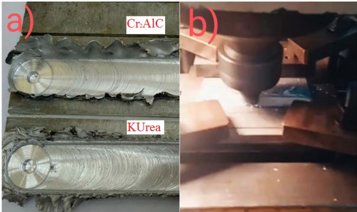
Figure 4.19: a) Result of FSP b) During the operation of FSP
