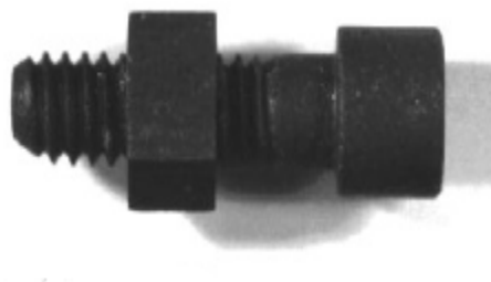
Figure 3.29: Screw-nut system machined from \text{Ti}_3\text{SiC}_2
