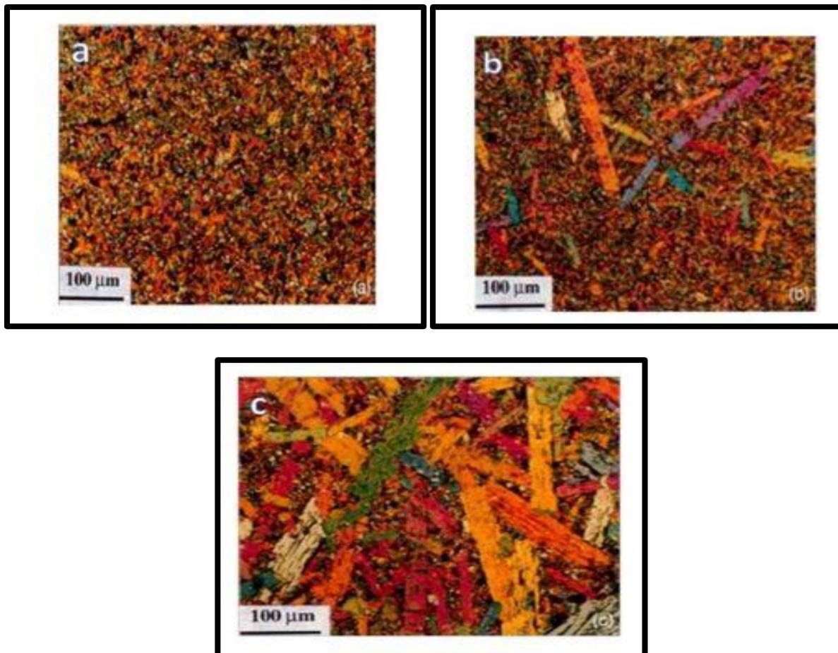
**Figure I. 4: Observation optique du Ti<sub>3</sub>SiC HIP 1450°C (a) Structure FG t=8h (b) structure CGFG t=16h (c) structure CG t=24h [15].**
