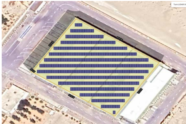
Figure IV.4: A design for the PV system on the roof of Frigomedit “Trifaoui”
