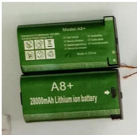
Figure III.11: Batterie 28000mah Lithium ion
