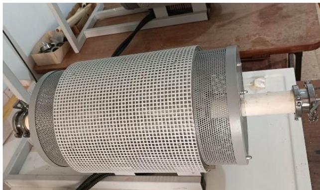
Figure II.6: Four tubulaire de marque CARBOLITE
