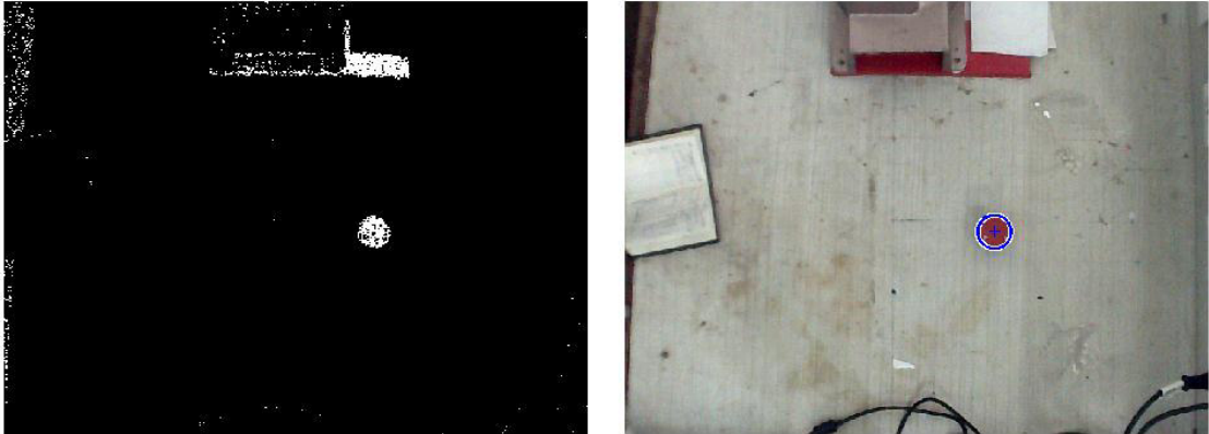
Figure (4.16): circle detection after thresholding and applying circle Hough transform
