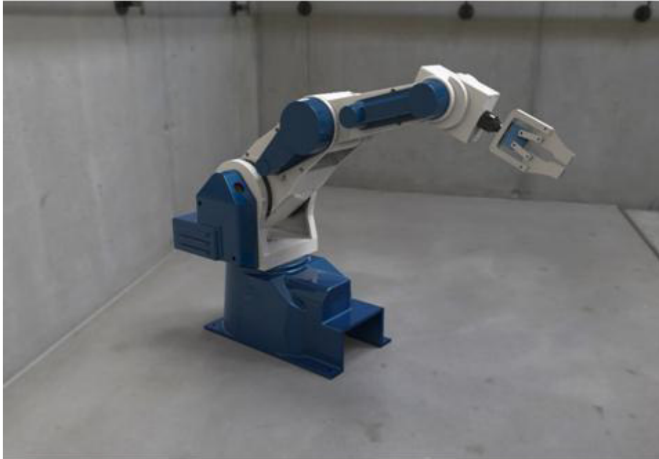
Figure 1: CAD model of IR50P robot manipulator
