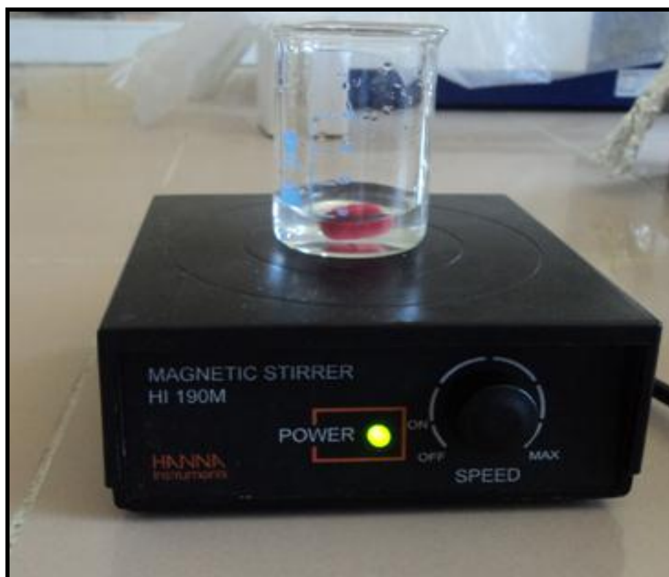
Figure 22 : Agitateur (Magnetic Stirrer HI 190M)
