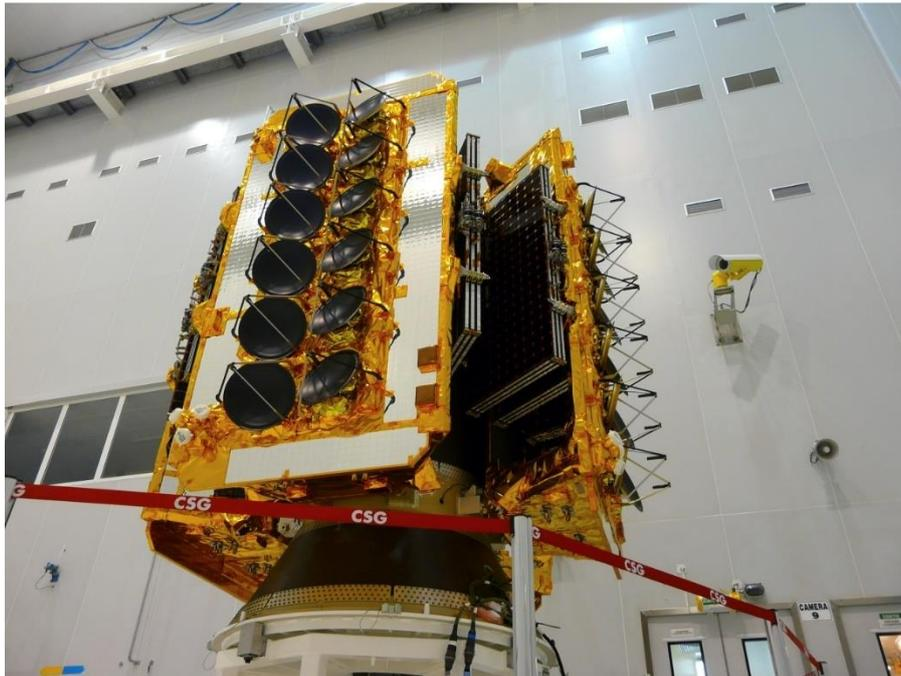
Figure 1-15 : charge utile du MEO (o3b) satellite Components – Photo [18].
