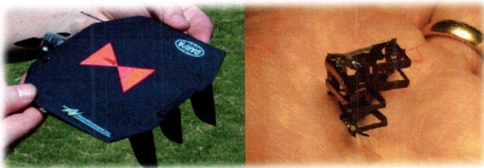
Figure 1.05 – Micro drones . Black Widow (Aerovironment, 42g) et Micromechanical FlyingInsect (UC Berkeley, 25mm)
