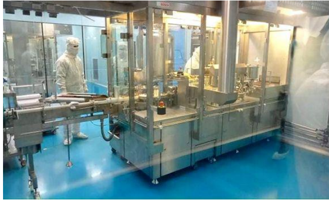
Figure 97: Dosing machine inside the controlled atmosphere area.
