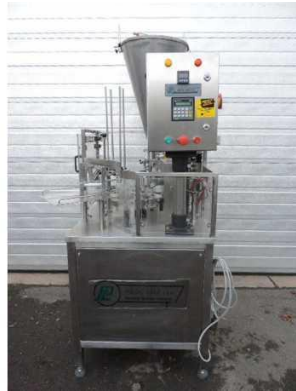
Figure 90: Hitimon dosing machine.
