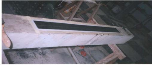
Fig.1 - Laminated plate located in the beam.
