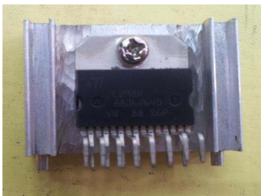
Figure 4.12 le circuit L 289 (pont H).
