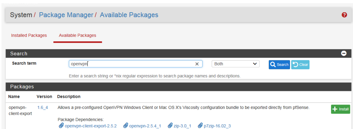
Figure 4.36 - Installation du package openvpn-client-export .
