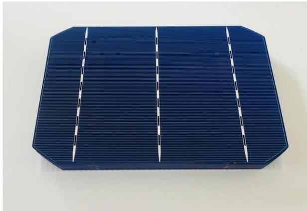
**Figure II.11 :** Plaque de silicium monocristallin.
