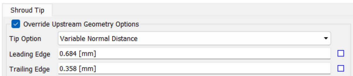
Figure III.3.10. Specifying the Radial Gap.
