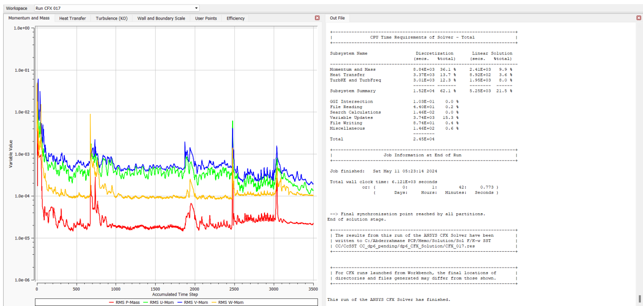
Figure III.5.14. View of the Ansys CFX Solver program window during the solution process.
