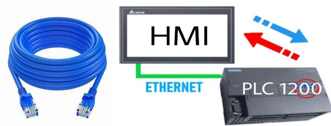
**Figure 4.4** Communication HMI/PLC.
