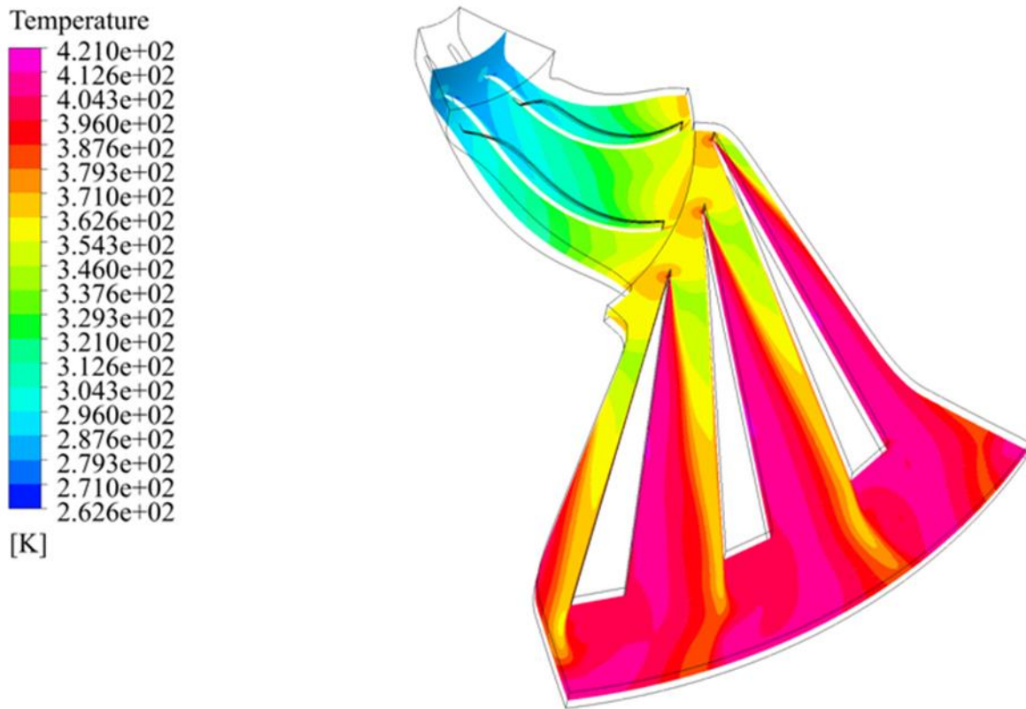
Figure 4-9 Relative Static temperature distribution in the blade-to-blade plane (RANS).
