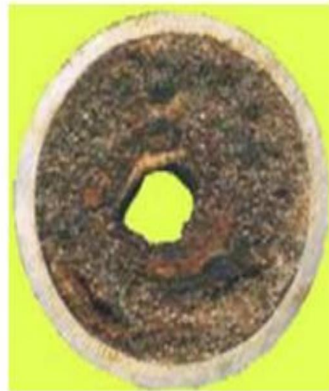
Figure 2-9: Wax deposition plugs in the wellbore on platform
