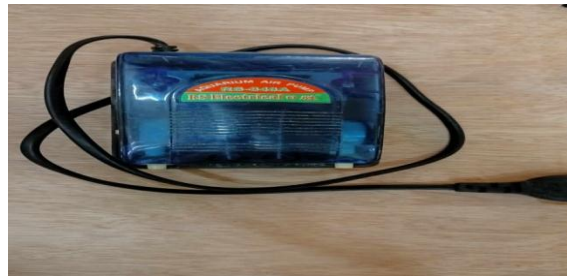
Figure 3-6 pompes a air.
