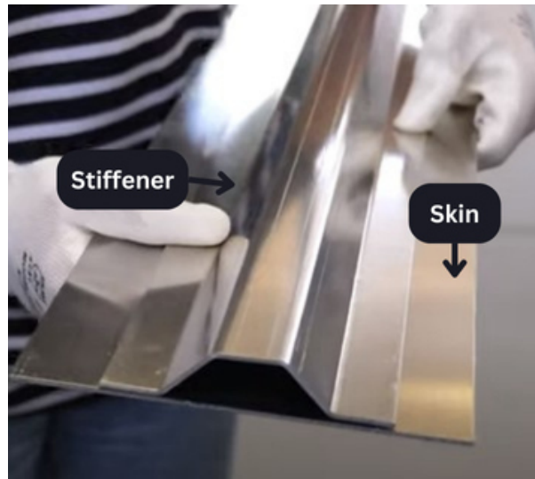
Figure 1.4. Aluminium Skin and Stiffener before welding [19]
