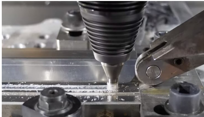
Figure 1.5. Stiffened panel during Lap Welding process [19]
