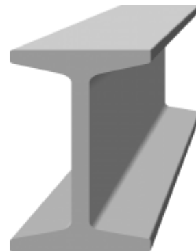
Figure 96: poutre IPE source : google image
