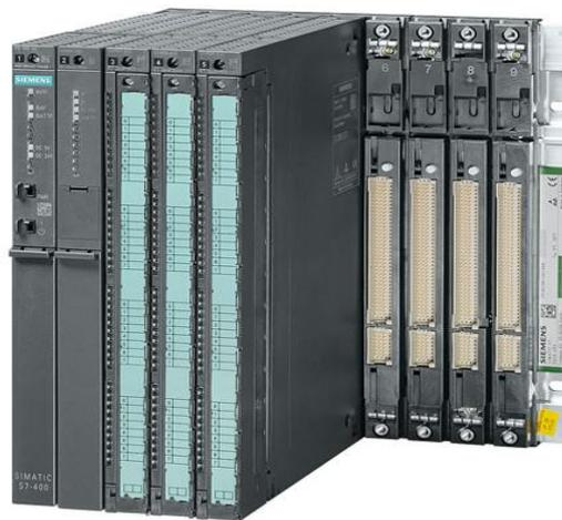
**Figure 3.6** *Automate programmable industriel (API) S7-400.*
