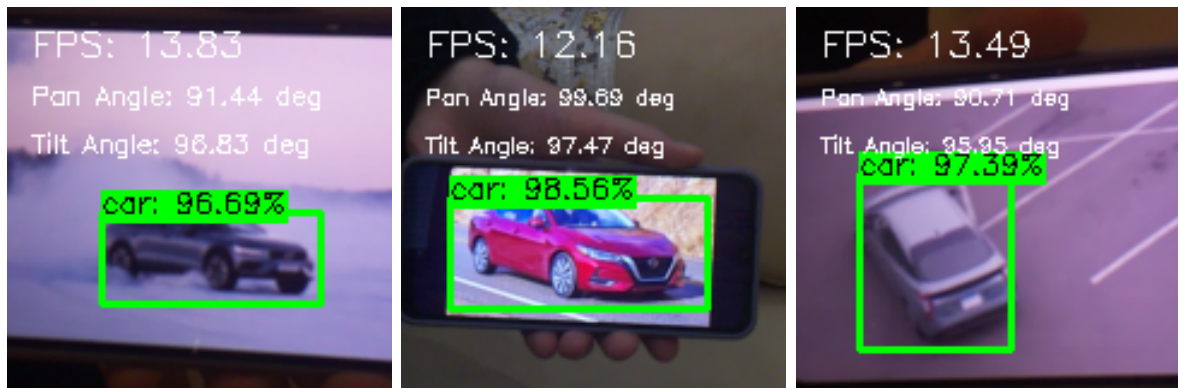
Figure III.33: Detection results using MobileNet SSD at a resolution of 160 \times 160 pixels.
