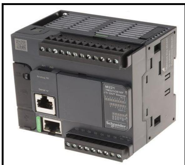
Figure. III .1 : L'Automate programmable Industriel (API)
