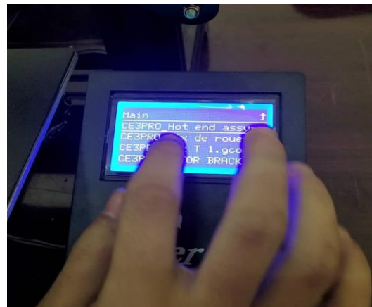
Fig 4.37: Select the part, then set the bed and extruder temperature.
