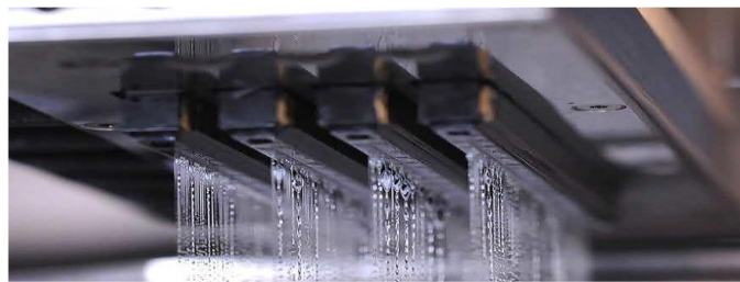
Figure 1.10 binder jetting technology in Action.
