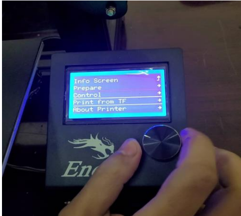
Fig 4.37: Select the part, then set the bed and extruder temperature.
