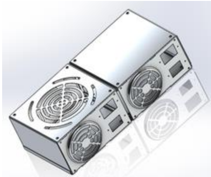
Figure 18 Cooling Unit 3D Model
