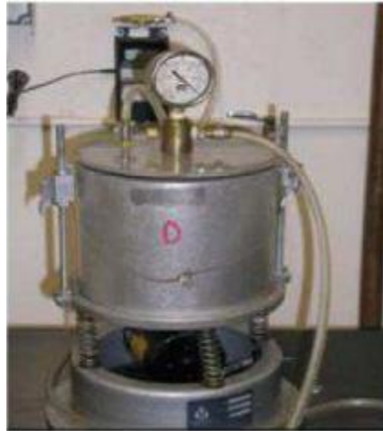
Figure I. 12: Vacuum Water Absorption Measuring Apparatus (Mills Beale Et Al. 2009) [18]
