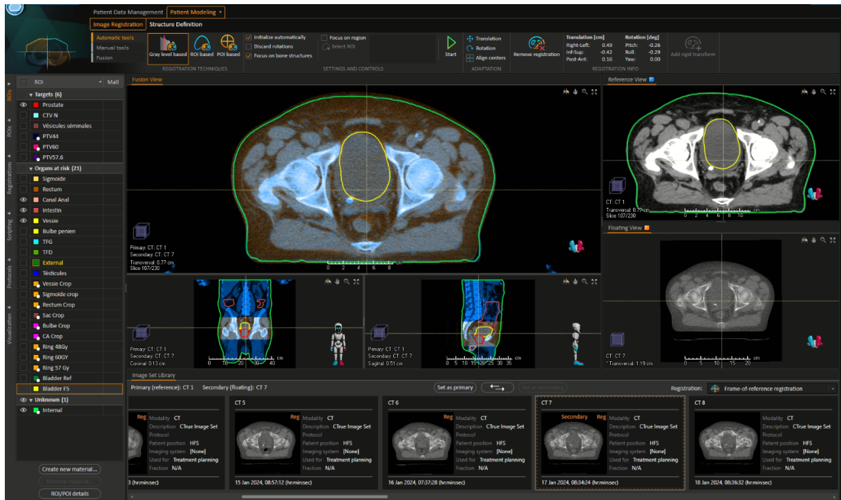
Figure 3.7: Image registration procedure between kVCT and MVCT scan images in RayStation™
