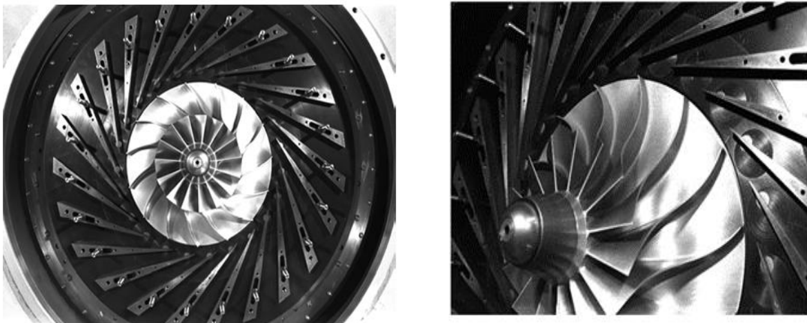
Figure 1.7 Centrifugal compressor stage - front wall removed [3]
