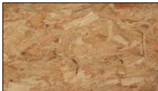
Figure 91: Aspect d’un panneau OSB, google image
