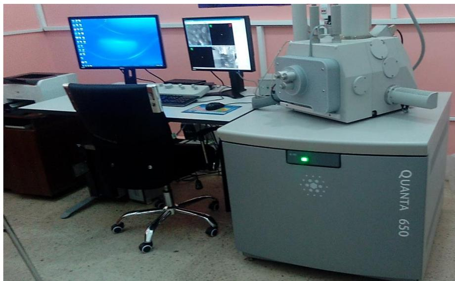
**Figure I.7.** Le MEB/EDX Quanta 650
