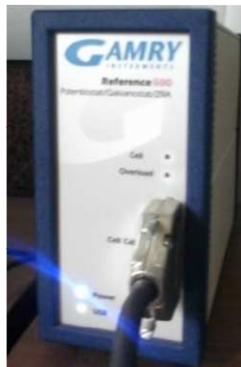
Figure IV.1: Potentiostat/Galvanostat de type GAMRY Ref 600.
