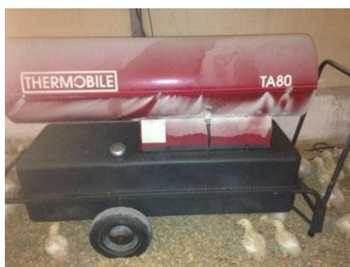
Figure 14: Chaudière à gazoil thermobile
