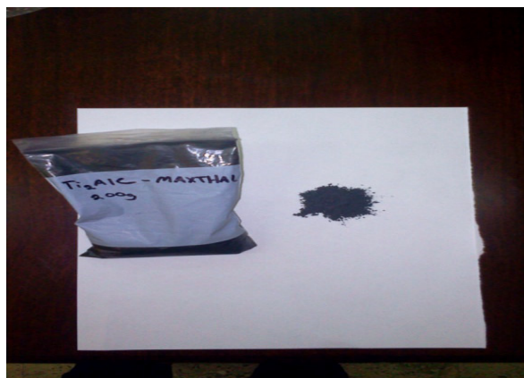
Figure III.1: Poudre de Ti_2AlC (MAXthal 211).
