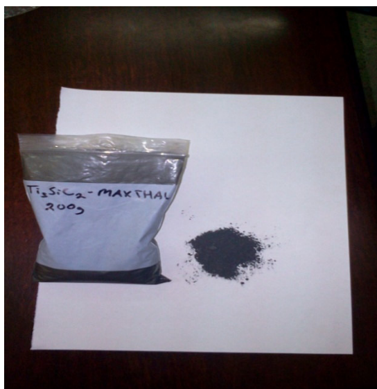
Figure III.2: Poudre de Ti 3 SiC 2 (MAXthal 312).
