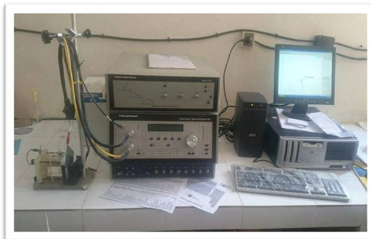
Figure 3.20: Potentiostat/Galvano stat EG&G 283
