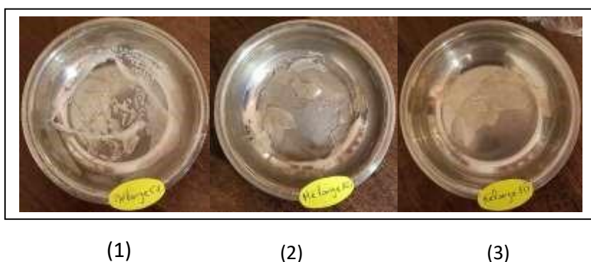
Figure II.1 : les films AC/PEVA "1" film de 5% AC, "2" film de 10% AC, "3" film de 15% AC.
