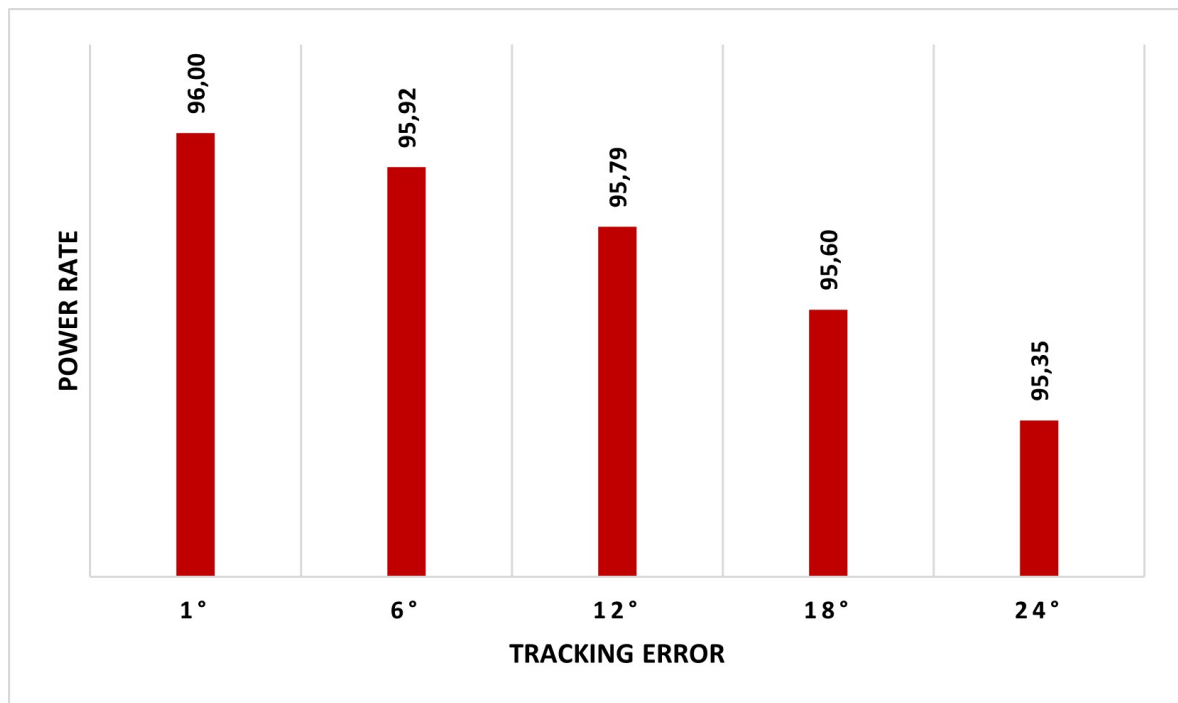
Figure 4.17: Generated Power Percentage for Different Tracking Error Percentages
