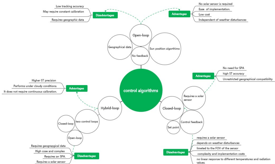
Figure 1.9: Control algorithms applied to solar tracking systems
