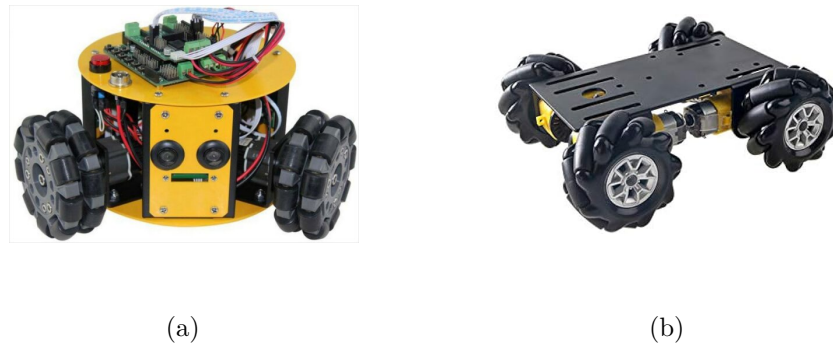
Figure. 1.12: Example of holonomic systems, (a) 3 mecanum wheeled robot, (b) 4 mecanum wheeled robot
