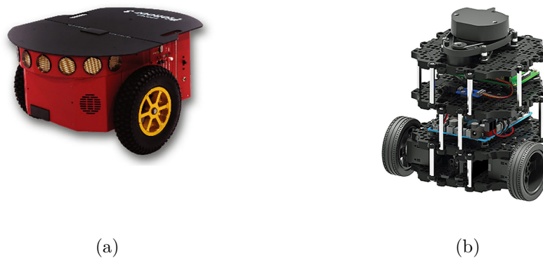
Figure. 1.13: Differential drive robots, (a) Pioneer 3DX model, (b) Turtlebot3 burger model.
