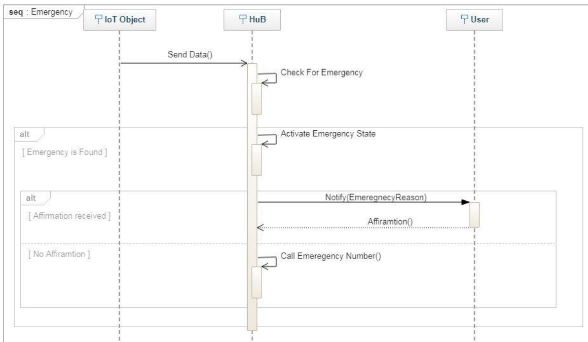
Figure 23 Sequence Diagram of Emergency.
