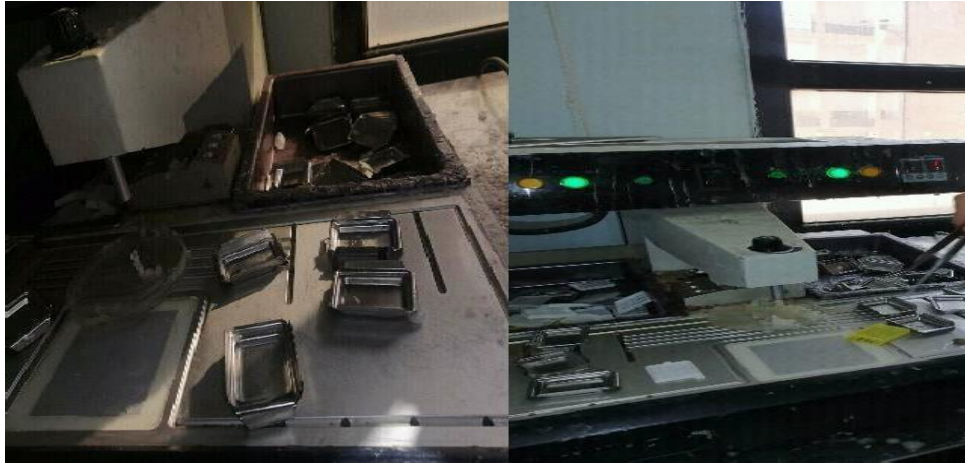
Figure 29: An automatic paraffin dispenser on the cassette (Personal photo 2024)
