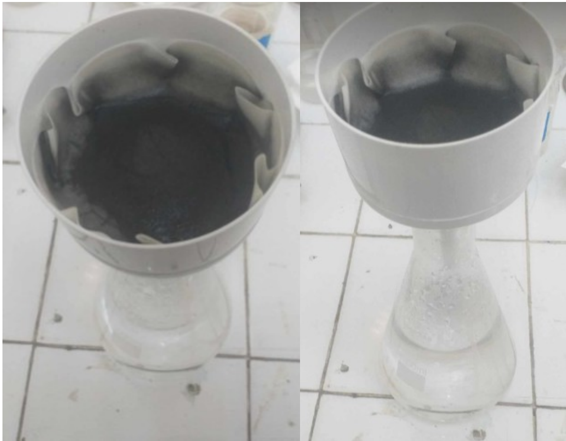
Figure II.16: the filtering/rinsing process tools (Conical flask/Erlenmeyer, filter, plastic funnel) - The next step is to put the filter in a Petri dish to be left in the laboratory oven until dry. The following figure shows the oven used to dry the powder.
