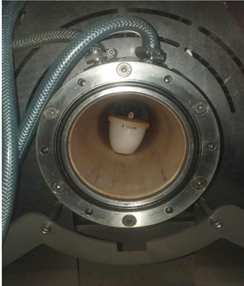
Figure II.12: sample inside the Tubular furnace Nabertherm GmbH 1800°C at C.R.T.I cheraga research Center.
