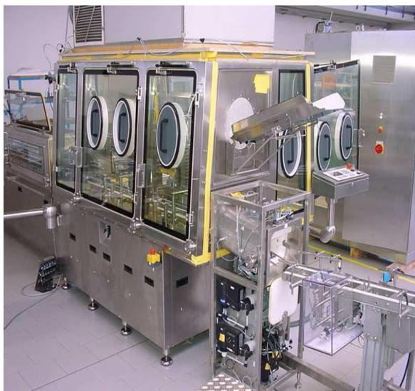
Figure 8: Photo isolateur rigide
