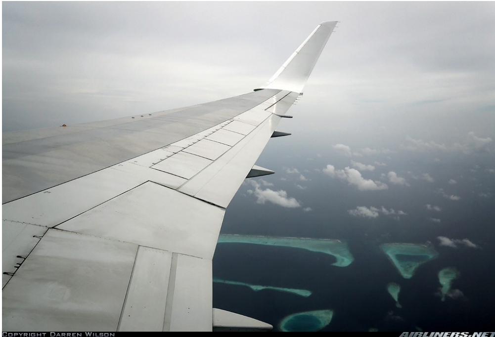
Figure II.2: Control surfaces exemplify well the use of plates structures in aeronautical engineering. Wing of Boeing 767-324. Image from www.airliners.net .
