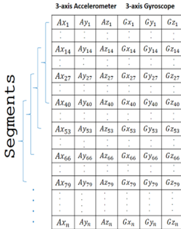
Figure 2. 15: Segmentation of sensors data with a 2 seconds and 66% overlap.
