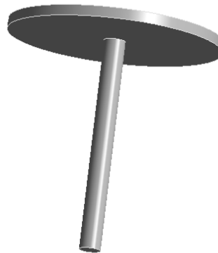
Figure II.12: Threaded steel rod grip.
