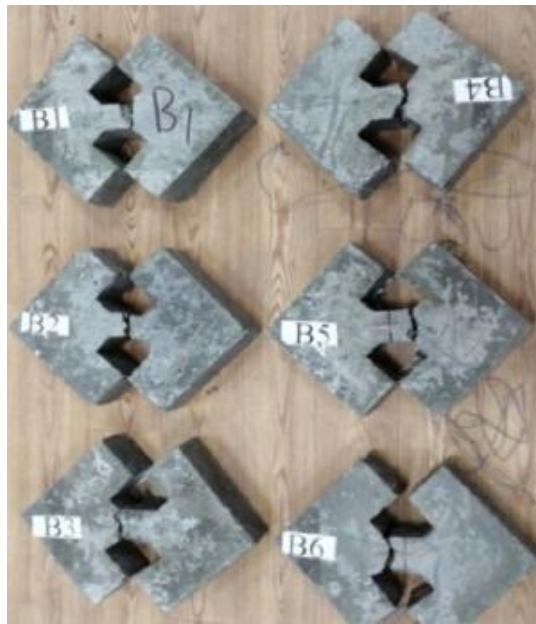
Figure I.26: Typical failure mode [108].
