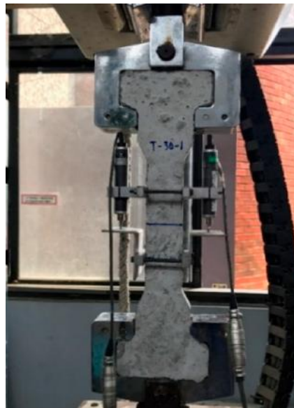
Figure I.15: Tensile test using lateral gripping method [93].
