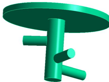
Figure II.8: Welded threaded steel rod grips.
