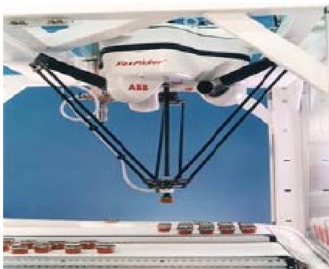
**Figure I.5 : Robot Delta. [3]**
