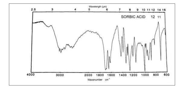
Figure 8. Absorption spectrum of Sorbic acid SCR.
