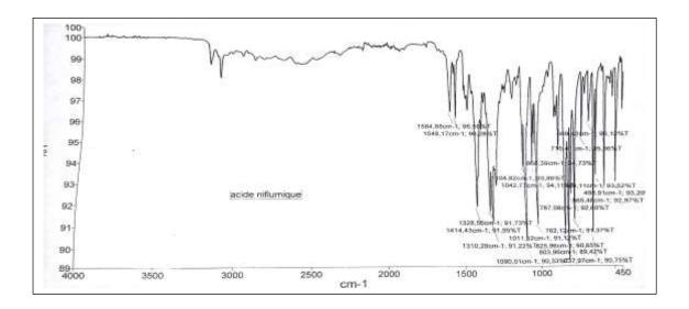
Figure 6.Absorption spectrum of Niflumic acid SCR.
