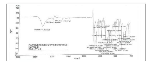
Figure 10. Absorption spectrum of Nipagine M Sodium SCR.
