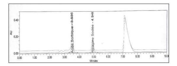
Figure 13.Chromatogram representing the excipients (Nipagine M Sodium, Sorbic Acid) in the test solution.
