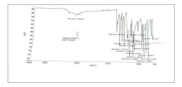
Figure 9. Absorption spectrum of Nipagine M Sodium (Test).
