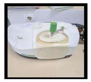
Infrared spectroscopy (IR)
