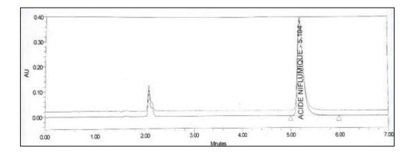
Figure 11.Chromatogram representing the dosage of the active ingredient (Niflumic Acid) in the test solution.
