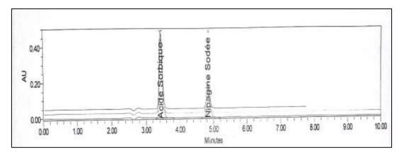
Figure 14.Chromatogram representing the dosage of the excipients (Nipagine M Sodium, Sorbic Acid) in the standard solution.
