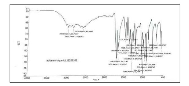
Figure 7. Absorption spectrum of Sorbic acid (Test).
