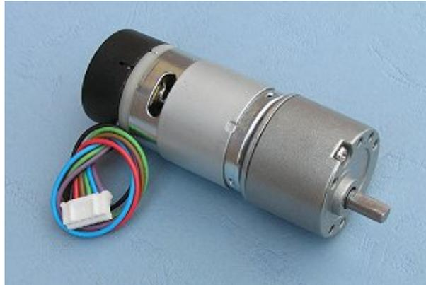
The EMG30 (encoder, motor, gearbox 30:1) is a 12v motor fully equipped with encoders and a 30:1 reduction gearbox. It is ideal for small or medium robotic applications, providing cost effective drive and feedback for the user. It also includes a standard noise suppression capacitor across the motor windings.
